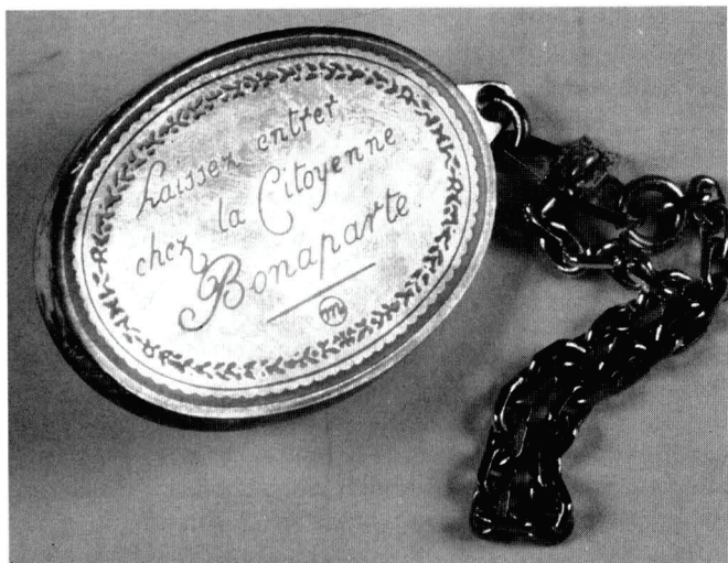
Figure 2. Tarnished silver-plated copper key ring. Continued cleaning of tarnish compounds will eventually remove the thin silver layer.
