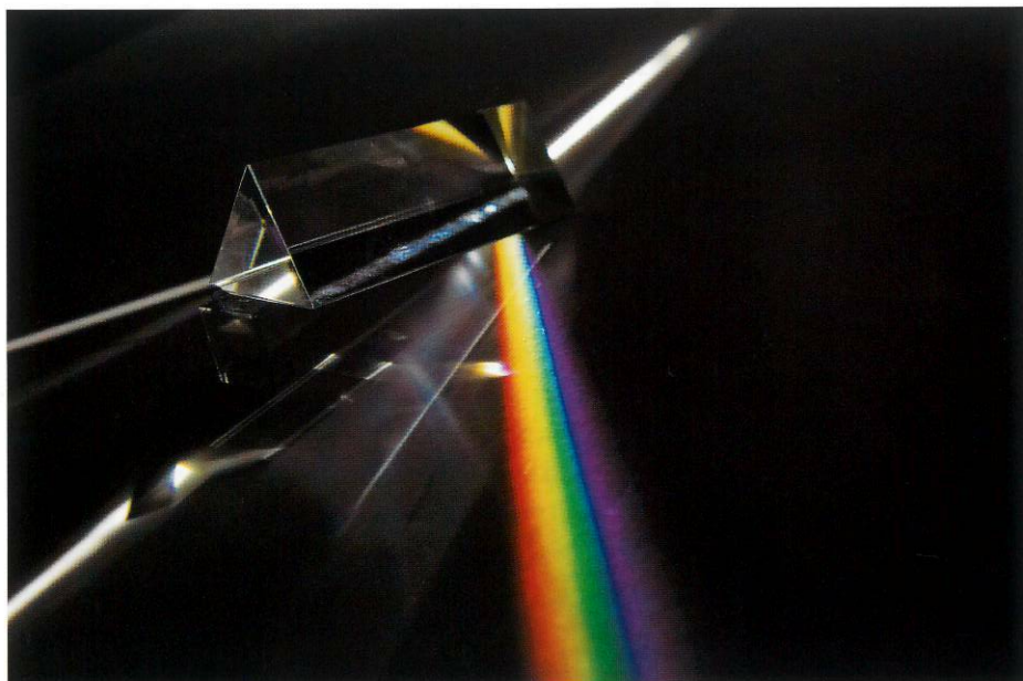
Figure 1.5. The classic demonstration—after Newton—that white light is composed of light of different wavelengths (colors).
